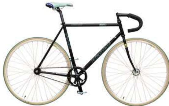
The construction of the track frame is similar to that of a road frame. The difference is in the geometry. Generally, the size of the track bike is the same as the road bike or slightly smaller, the bottom bracket is higher and the chain stays tend to be short. These characteristics make the track bike more rigid and responsive than the road bike.
